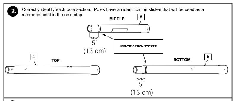
Bounce middle pole section (5) into top section (4) using a wood scrap as shown until the top pole no longer moves toward the pole identification sticker on the middle pole.
